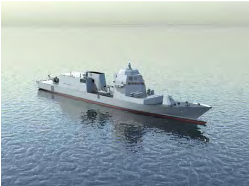
The seven frigate-sized PPA (Pattugliatori Polivalenti d'Altura – multi-purpose blue water OPVs) for the Italian Navy will be built in three different configurations, based on a common platform but with scaled combat systems.
