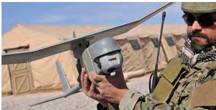
AeroVironment's RAVEN can be launched right from the hand of the soldier.
