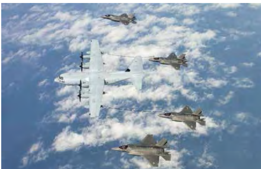
At present, there are 16 nations operating the C130J SUPER HERCULES airlifter. Shown here are two F-35Bs refuelling from a KC-130J tanker of the USAF.
